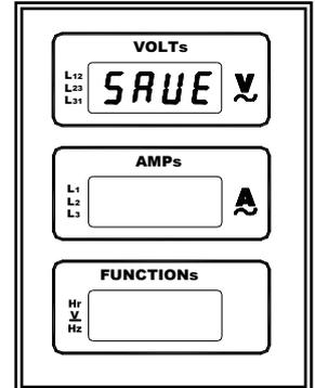
If the buttons are left untouched for 10 seconds, the operation terminates showing (END) on the screen and the control turning OFF and any modification made to the hour meter will not be recorded.
