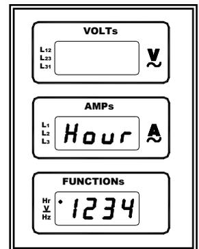
Press the UP and DOWN buttons to change the hours. By pressing and holding, you can speed up the process. When the setting is completed, press the (PEN) button for 4 seconds until (SAVE) appears on the screen.
