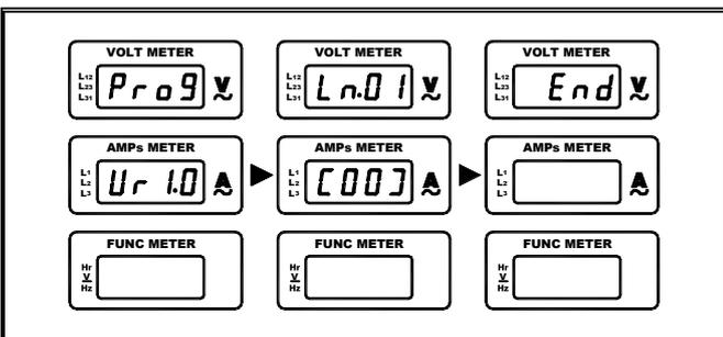
The GCU-100 comes pre-programmed with factory settings. You can reset to factory setting at any time by pressing the (UP and Down arrow) buttons together for 4 seconds until “Au.PO” appears on the screen.
