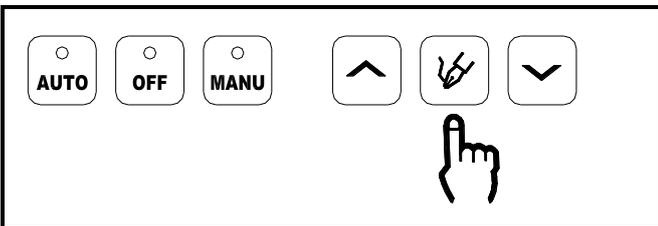
The display screen will now display “Prog” & “Vr1.0” for 4 seconds, “Vr1.0” is the program version. Next “Ln.01” will appear on the display screen, representing the program setting entry, (00) the system setting parameter.
