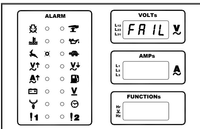
Some electronics speed controllers “Governors” do not share the MPU with other devices, so you may have to install another (MPU) or use a dual coil MPU with the GCU-100. When the control cannot read the frequency correctly, the GCU-100 shuts down the engine and the MPU failure icon lights up on the panel.
